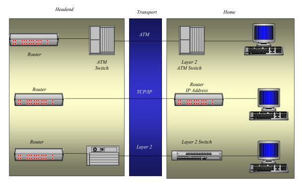
Both ATM and Ethernet have the same architectural elements; some central device, some filed unit for distribution, and some end user interface. However, the differences are significant:
