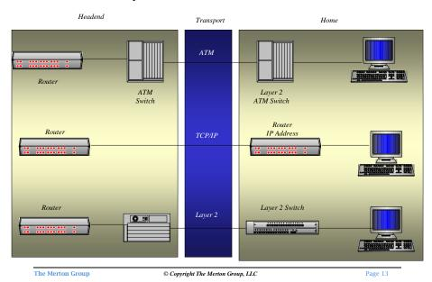
The difference between ATM and Ethernet is best shown below. They both have the same architectural elements; some central device, some filed unit for distribution, and some end user interface. However the difference are significant:
