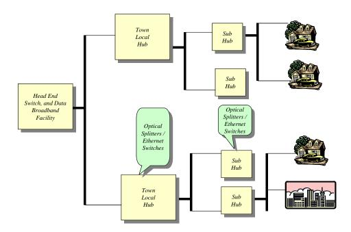
The basic architecture for local PON or Gigabit Ethernet is shown below. The elements are:
