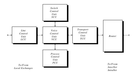
LCU: The Line Control Unit, LCU, is the interface between the telephone network and the IVN. The LCU provides for call initiation and termination. The initial LCU is a Dialogic card which provides for signaling to and from the local telephone network. The use of the Dialogic cards can be customized for each local market telephone interface elements.
