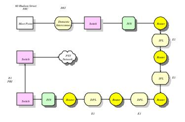
The network shown above originates in the U.S. and "lands" in multiple locations throughout Europe. It creates entry portals in all of the markets in which the Company operates. The network then "expands" in a country as shown below for Italy.
