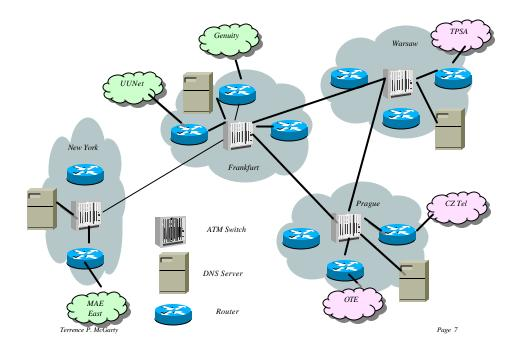
The overall architecture of the MAE Europe construct is shown below. It consists of NAPs which are interconnected as a distributed single entity. These NAPs then interface with other NAPs and MAE East and West, as may be required.
