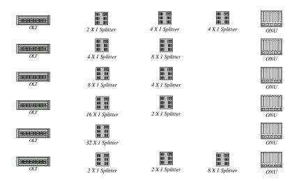
A typical design is shown below. It demonstrates 2 strands per OLT. It feeds a 32 strand fiber. Note that 96 strand fibers are readily deployed and the details will be left to the system engineer based on final strand mapping.
