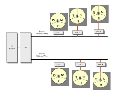
The above design shows that we need besides the fiber a set of small microcell BSCs as well as antenna. These are the additional elements.
