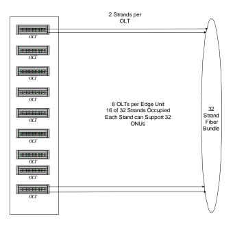
A typical build out is shown below. This time distance are also applied. This will appear as a hybrid active/passive design. The passive side is per town and this minimizes operations and maintenance costs. The active side is in one enclosed unite per town. The active equipment per town takes not more than 150-250 sq ft areas and can be readily housed in local space.
