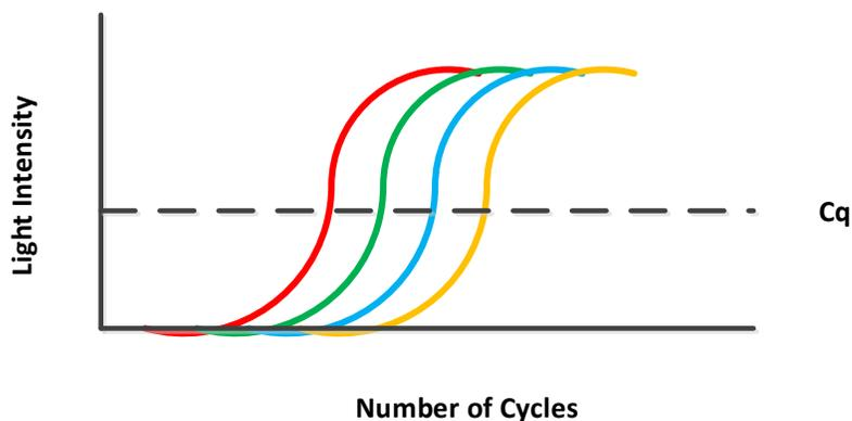
A key factor is the  $C_T$  value. We use this as a baseline to measure the intensity depending on PCR cycles.
