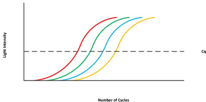
Note: A cycle is a temperature/doubling cycle. Thus we start with 1, then 2, then 4, 8, 16 etc. Each is tagged with a fluorescent and they grow in number until they can be readily seen and measured in intensity. Each of the above curve is for a different miRNA
